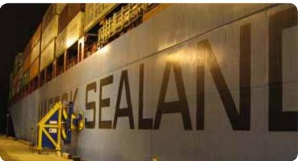
Oman's Port of Salalah installed two MoorMaster™ 400 units at a container berth on a trial basis in September 2005. The six-week trial was designed to measure the MoorMaster™ system's ability to reduce the surge motion caused by 'long waves' on container
