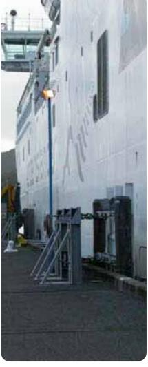
The very first MoorMaster<sup>™</sup> automated mooring system, the MoorMaster<sup>™</sup> I-400, was installed on the rail passenger ferry Aratere in 1997. The Aratere has an LOA of 150 metres, and 12,000 tonnes displacement. Four MoorMaster<sup>™</sup> units are positioned on the vessel,
