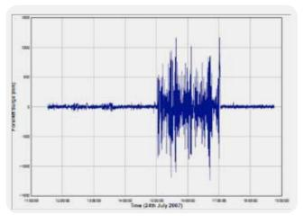
MoorMaster™ automated mooring systems are in use at the Port of Salalah at two of the port's six container berths, where they moor vessels of up to 362m LOA. The most recent installation has a holding force of 2,400 kN, provided by 12 x MM 200 units. The primary reason for the Port of Salalah to use vacuum mooring is to dampen
