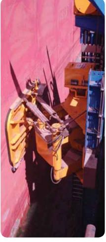
Fourteen MoorMaster™ MM200 units, with a total capacity of 2,800kN, spaced at 14m intervals, are installed at Port Hedland in Western Australia. The MoorMaster™ units moor dry bulk carriers of up to 135 kdwt, 295m LOA.
